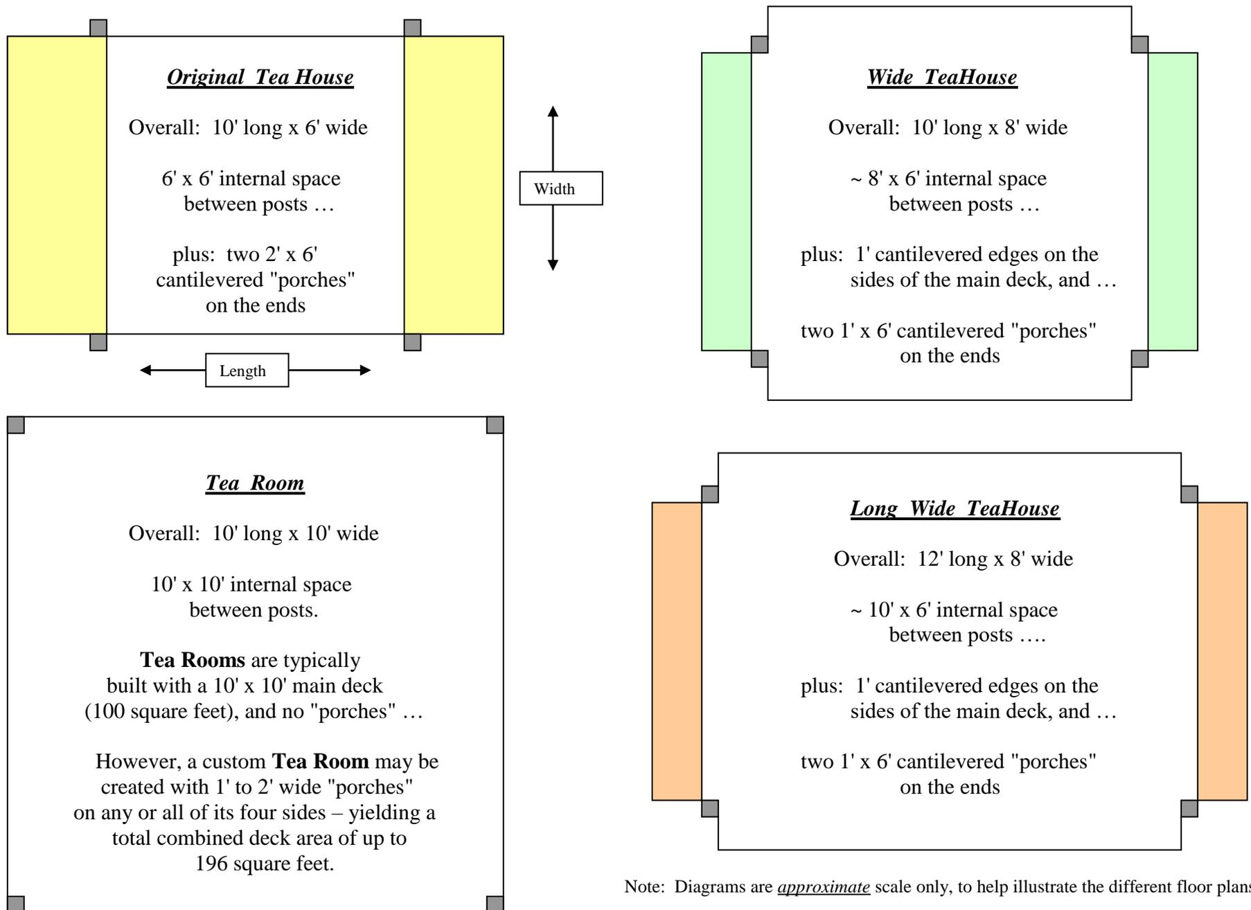
Note: Diagrams are *approximate* scale only, to help illustrate the different floor plans.
